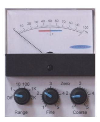
•Ranges: x1, x10, x100, x1000, x2000 •Sensing plate area: •Tube setting **2.25** sq. in. metal plate (included) sqlass tube (included) •Plate setting **2** sq. ft. metal plate •Sensor connectors: standard banana jack •Recorder output: 0 -2.5V standard 1/8" mono phono jack •Power: 4 "AA" batteries (included) •Sensing distance ie. human body
